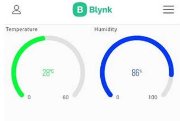
Fig. 5. Temperature and humidity display on Blynk application
