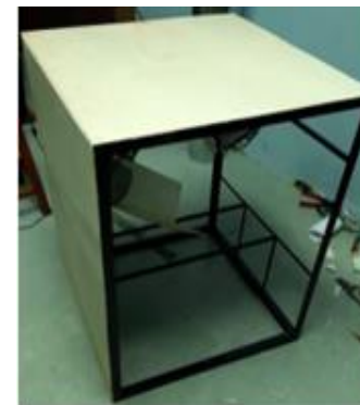
Fig. 10. Installing the plywood to the frame
