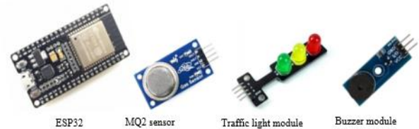
Fig. 2. Gas leakage detector component
