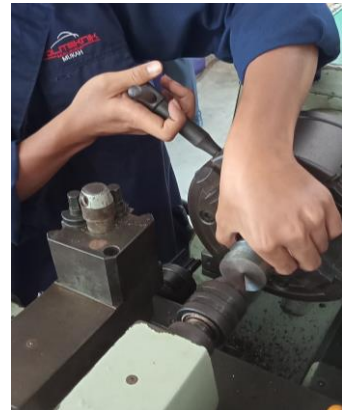
Fig. 2. Existing tightening process (without jig)
