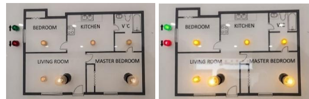
Fig. 13: Light dimming control and shutter position control
