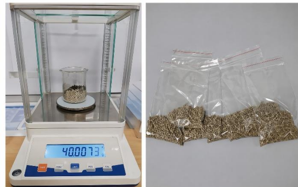
Fig. 3: The mixing process of PLA with NF (a), a weighted composite total of 40 g, and (b) packing in a small zip-lock bag
