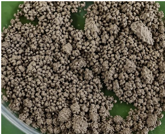
Fig. 2: Structure of PLAF after the sieving process
