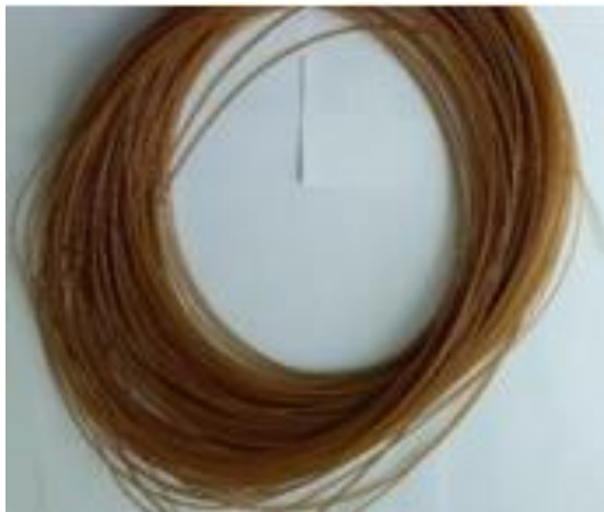
Fig. 6: The composite filament produced after the extrusion process PALF/PLA
