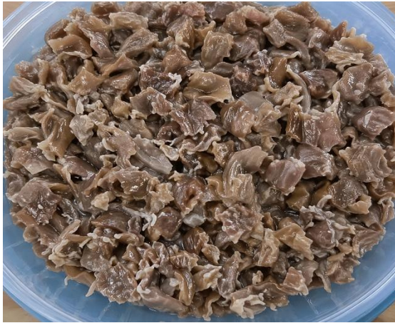
Fig. 5: The structure of composites after the crushing process, PALF/PLA
