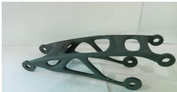
Fig. 17: Illustrates the prototype done for 3D printing
