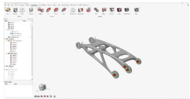
Fig. 10: Illustrates the optimized geometry, which was subsequently refined to produce a manufacturable prototype
