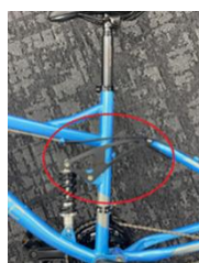
Fig.1: MTB rocker arm to enhance its stiffness
