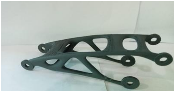
Fig. 17: Illustrates the prototype done for 3D printing
