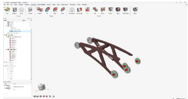
Fig. 9: Illustrates the TO conducted to minimize weight and improve stiffness while preserving structural integrity
