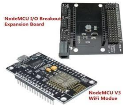
Fig. 3: NodeMCU V3 development board with integrated Wi-Fi
