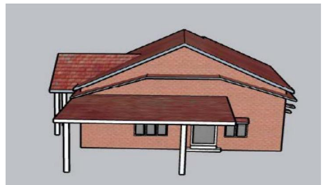
Fig. 3: 3D SketchUp model of the same building created from combined UAV and mobile LiDAR data, meeting LOD 3
