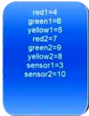
Fig. 2. The output pins from Arduino that have been used
