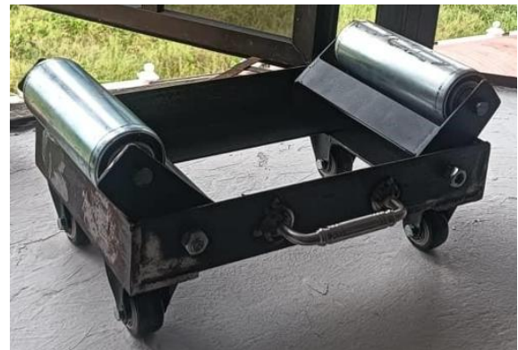
Fig. 5: Fabrication of Foldable Tire Changer
