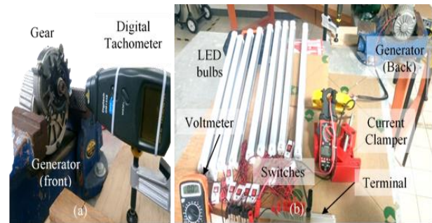
Fig. 4. Load-condition setup with the 12 V system
