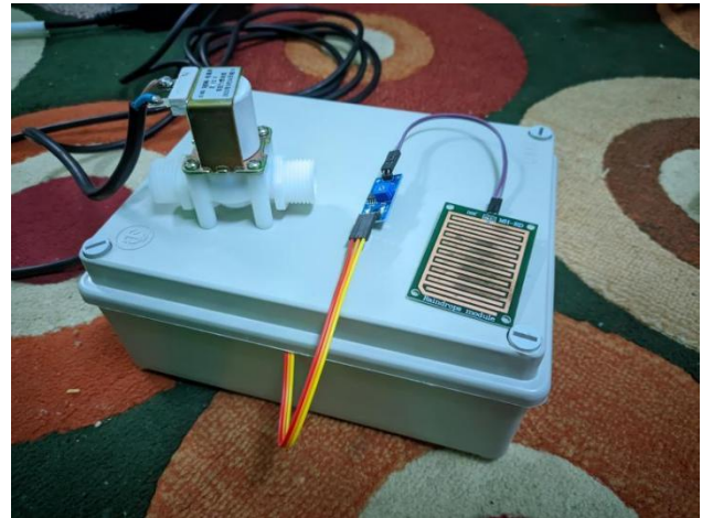
Fig. 4. Photograph of the complete RHS prototype
