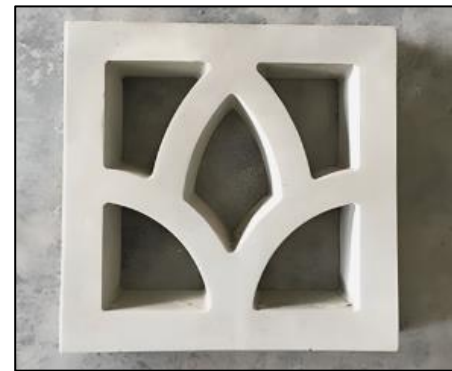
Fig. 17. Breeze block reinforced with nipa palm leaf ash
