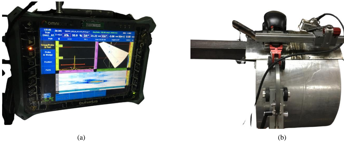
Fig. 1 (a). Ultrasonic flaw detector, and (b) the scan plan set up on a steel pipe
