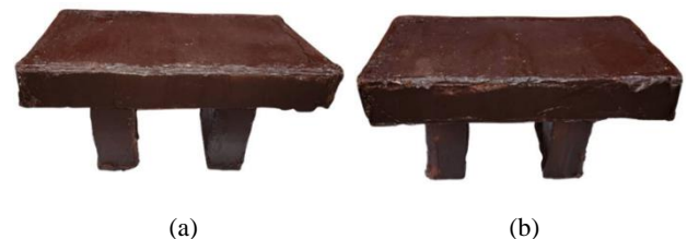
Fig. 4. Table made from drink cartons and natural fibre (a) sugarcane bagasse (b) banana stem
