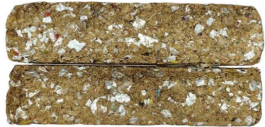
Fig. 3. Block made from drink cartons and paddy husk
