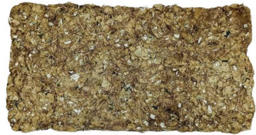
Fig. 2. Block made from drink cartons and banana stem
