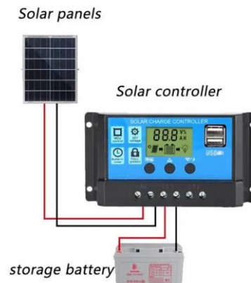
Fig. 9. Solar panel with PWM solar charge controller
